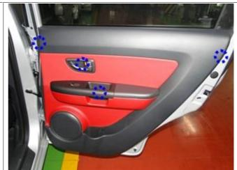
2) Disconnect the power window connector (B) and remove the door trim panel.
