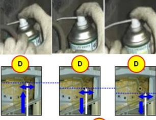
1.3.2 Push the nozzle tip deeper into the side member to apply wax evenly throughout the panel as shown in the photo (E). Spray the cavity wax by moving the nozzle tip back and forth and right and left.
