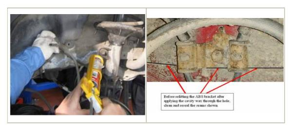
The images above show the area for resealing, use a wire brush to clean the existing sealer and surrounding area of any dirt and debris. Apply new sealer and stone guard as shown in the images both above in 3.1 and below in 3.1.2 and 3.1.3
