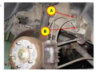
1.3 Spray the cavity wax onto the inside (bottom panel) of the rear floor side member through the wheel guard fastener hole using the spray lance (C) supplied, according to the procedure described in 1.3.1 to 1.3.3 below.
