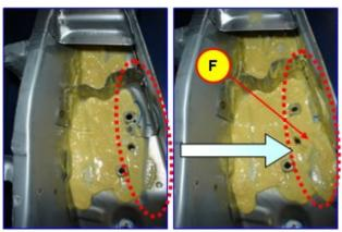
2. Spraying Cavity Wax onto the Inside of Rear Floor Cross Member 120ml.
