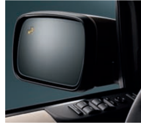
Blind Spot Monitoring* uses side-mounted radar to warn of vehicles in the driver's blind spot. A bright amber warning icon is illuminated in the appropriate door mirror when a hazard is identified.
