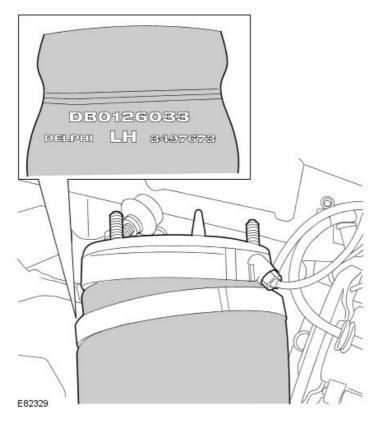
2. Renew the front air spring where necessary. For additional information, refer to Range Rover (LM) Workshop Manual Section 60 - FRONT SUSPENSION, Air spring assembly (60.21.01).
