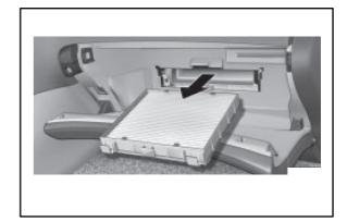
7. Remove the filter from the filter case.
