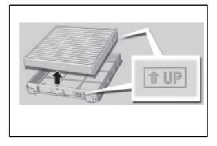
8. Install the NEW filter and reassemble in reverse order of disassembly.
