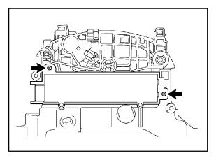
3. Remove the original shift lever anti–rattle cushion and replace with the new part, as shown in the illustrations.
