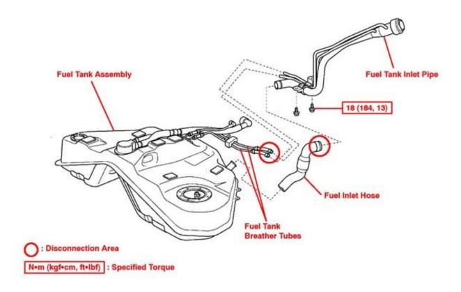
Fig. 2: Removing Fuel Tank Inlet Pipe Sub-Assembly
