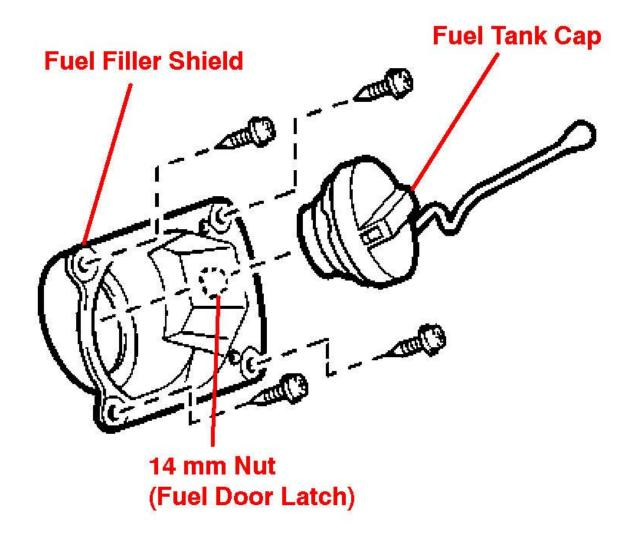
Fig. 1: Removing Fuel Filler Shield
