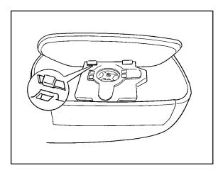
Repair Procedure (Continued) E. Reconnect the mirror holder — Apply pressure to the indicated areas until you hear the holder clips snap into place.
