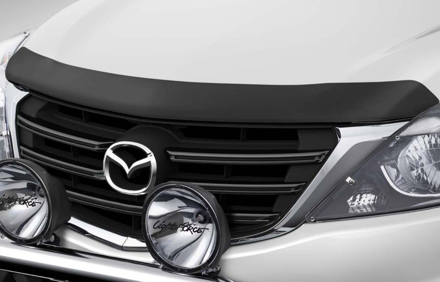
MATTE BLACK BONNET PROTECTOR Keep your paintwork safe from chips and dents.
