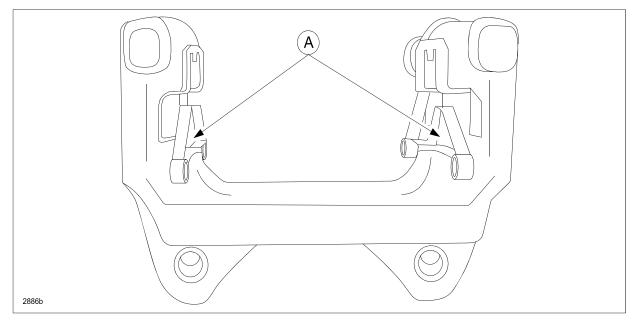
2. Using a wire brush, remove all rust from the rear brake caliper support area (A) until the surface turns glossy (B).
