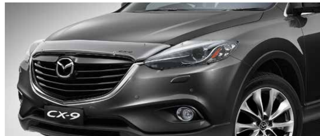
Bonnet protector (clear) Guards against damage from stones and other debris.
