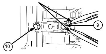
10. While holding cam cap number 4L in the shifted position, torque fasteners number 9 (inboard) first, to 8 Nm (72 lb-in), then torque fastener number 10.
