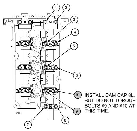
9. Using a screwdriver positioned on each side of the top of cam cap number 8L, apply hand pressure and shift the cam cap toward the **EXHAUST** side of the cylinder head.
