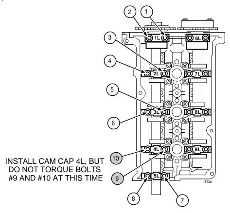
9. Using a screwdriver positioned on each side of the top of cam cap number 4L, apply hand pressure and shift the cam cap toward the **EXHAUST** side of the cylinder head.
