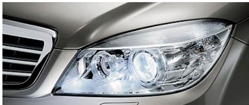
Intelligent Light System with bi-xenon headlamps
