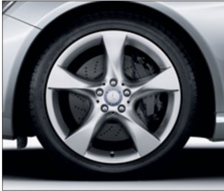
5-spoke light-alloy wheels with 255/40 R 19 front and 275/40 R 19 rear tyres, 255/40 R 19 tyres all round on 4MATIC models (optional)
