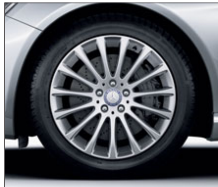
15-spoke light-alloy wheels with 255/45 R 18 front and 275/45 R 18 rear tyres, 255/45 R 18 tyres all round on 4MATIC models (optional, standard for CL 500 4MATIC BlueEFFICIENCY)
