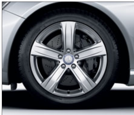
5-spoke light-alloy wheels with 255/45 R 18 tyres all round (standard for CL 500 BlueEFFICIENCY)
