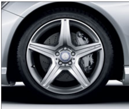
5-spoke AMG light-alloy wheels with 255/40 R 19 front and 275/40 R 19 rear tyres, 255/40 R 19 tyres all round on 4MATIC models, high-sheen finish (AMG Sports package)
