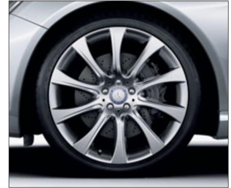
10-spoke "Alaraph" light-alloy wheels with 255/35 R 20 front and 275/35 R 20 rear tyres, 255/35 R 20 tyres all round on 4MATIC models, sterling silver (ex-factory accessories)
