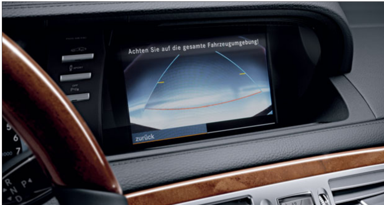
All-round visibility when parking and reversing – thanks to the optionally available reversing camera
