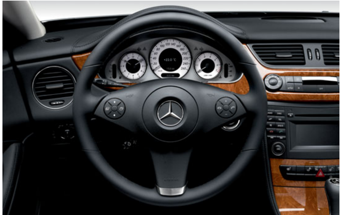
The multifunction steering wheel allows the driver to use the telephone and the radio as well as to navigate through various vehicle functions in the instrument cluster display while keeping both hands on the wheel
