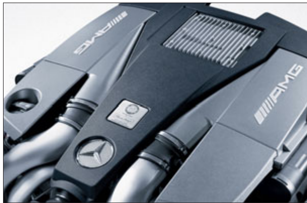
Tried-and-tested technology: the AMG 5.5-litre V8 engine with biturbocharging.
