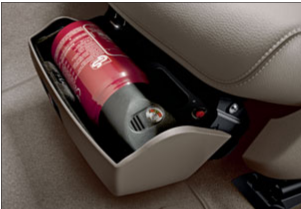
Fire extinguisher, mounted at the front of the driver's seat.
