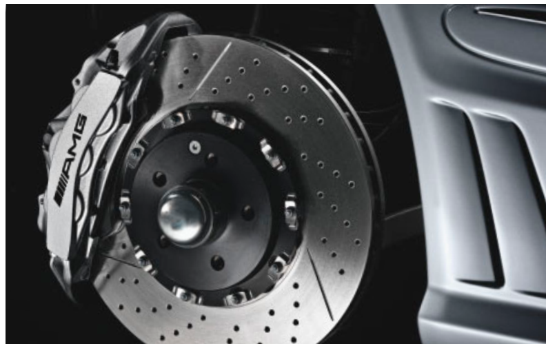
AMG braking system with composite brake discs
