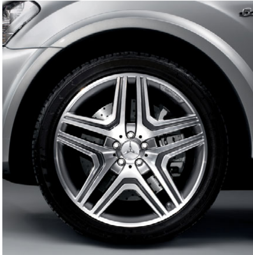
High-shine 5-spoke AMG light-alloy wheel with 295/35 R 21 tyres, painted in titanium grey (optional for ML 63 AMG)
