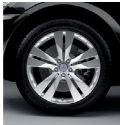
5-spoke light-alloy wheel with 265/45 R 20 tyres 3
