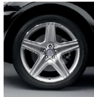
5-spoke light-alloy wheel with 265/40 R 21 tyres 4
