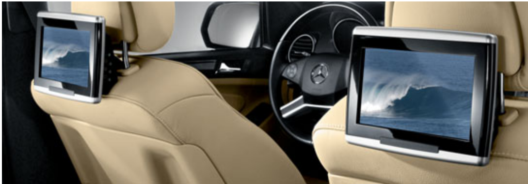
The Rear Seat Entertainment System with two screens in the front head restraints
