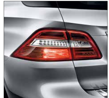
Tail lights featuring LED fibre-optic technology.
