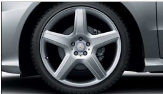
5-spoke AMG light-alloy wheel with 265/40 R 21 tyres (optional, Code 777)
