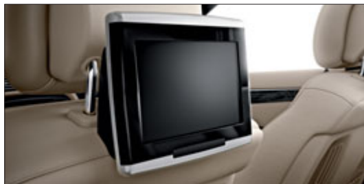
The two displays for the Rear Seat Entertainment System are mounted on the front-seat head restraints
