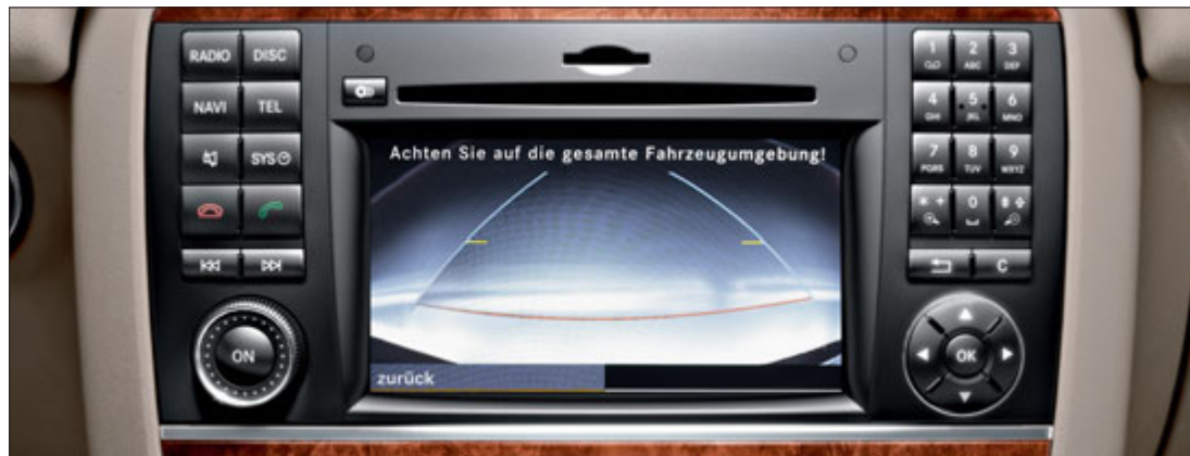
The reversing camera films the area around the tail end of the car
