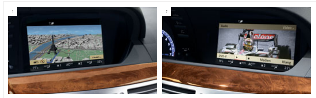
SPLITVIEW displays two different images at the same time – for the driver (1) and front passenger (2) – on a single screen
