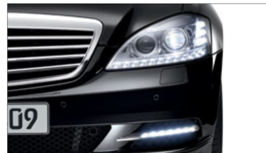
LED Light package: Intelligent Light System and LED daytime driving lights in the bumper
