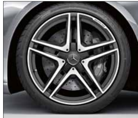
AMG 5-twin-spoke forged wheel, painted in titanium grey and polished, with 255/40 R 20 front tyre and 285/35 R 20 rear tyre (only for S 63 AMG, S 63 AMG 4MATIC and S 65 AMG, Code 753).
