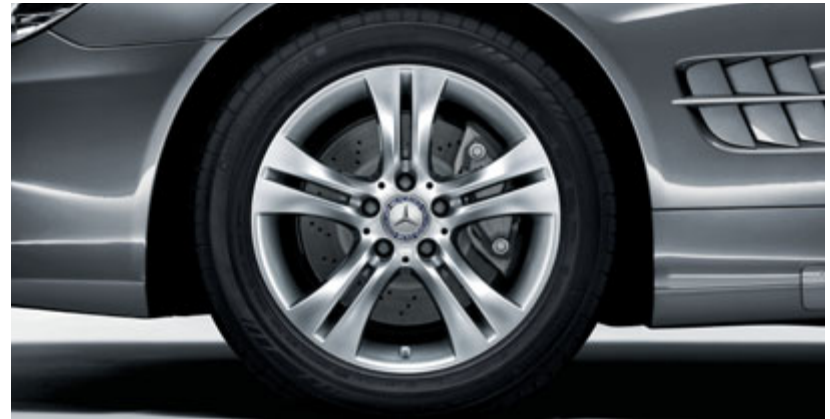
5-twin-spoke light-alloy wheels with 255/45 R 17 tyres (standard for SL 350)
