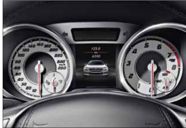
Instrument cluster with display with TFT technology.
