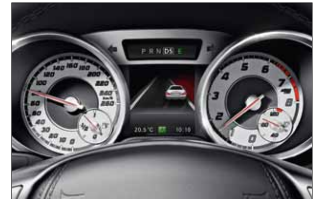
The Lane Keeping Assist warns the driver by vibrating the steering wheel if the car moves out of the lane unintentionally.
