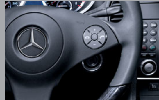
The multifunction buttons allow you to control many of the COMAND APS system's functions directly from the steering wheel
