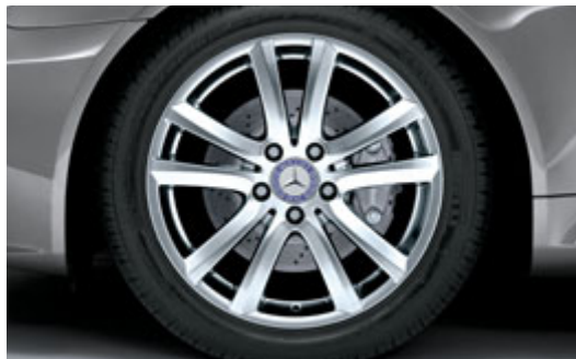
"Kikuchi" 5-twin-spoke light-alloy wheel with 225/45 R 17 tyres at the front and 245/40 R 17 at the rear
