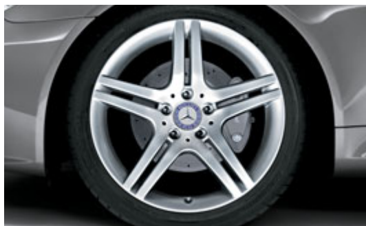
5-twin-spoke light-alloy wheel, titanium silver, with 225/40 R 18 tyres at the front and 245/35 R 18 at the rear (only in conjunction with Sports package)
