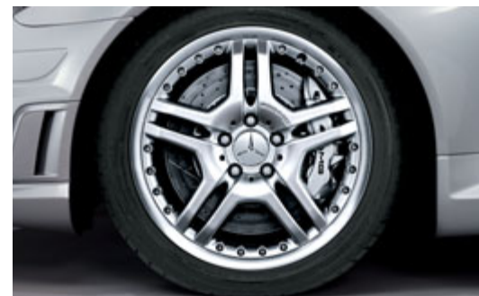
AMG twin-spoke light-alloy wheel, multi-piece, with 225/40 R 18 tyres at the front and 245/35 R 18 at the rear (optional for SLK 55 AMG)
