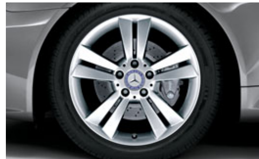
5-twin-spoke light-alloy wheel with 225 / 45 R 17 tyres at the front and 245 / 40 R 17 at the rear (standard for SLK 350, optional for SLK 200 KOMPRESSOR and SLK 300)
