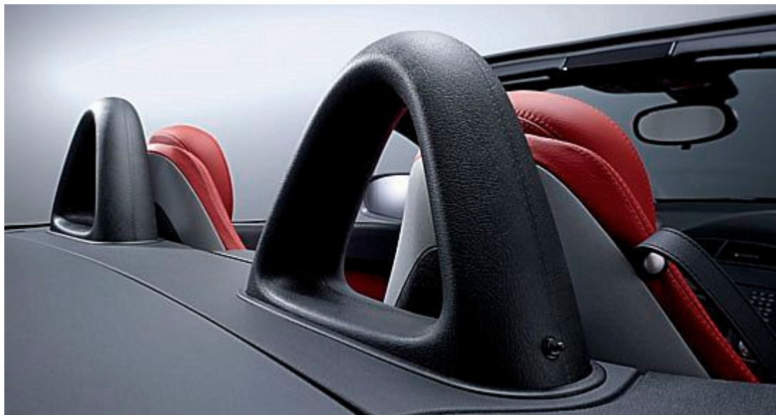
The roll-over bars offer added protection if the worst comes to the worst
