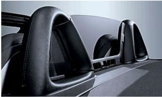
The perspex draught-stop reduces airflow turbulence
