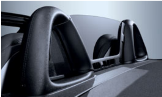
The perspex draught-stop reduces airflow turbulence
