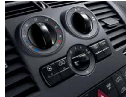
Air conditioning (TEMPMATIC).
