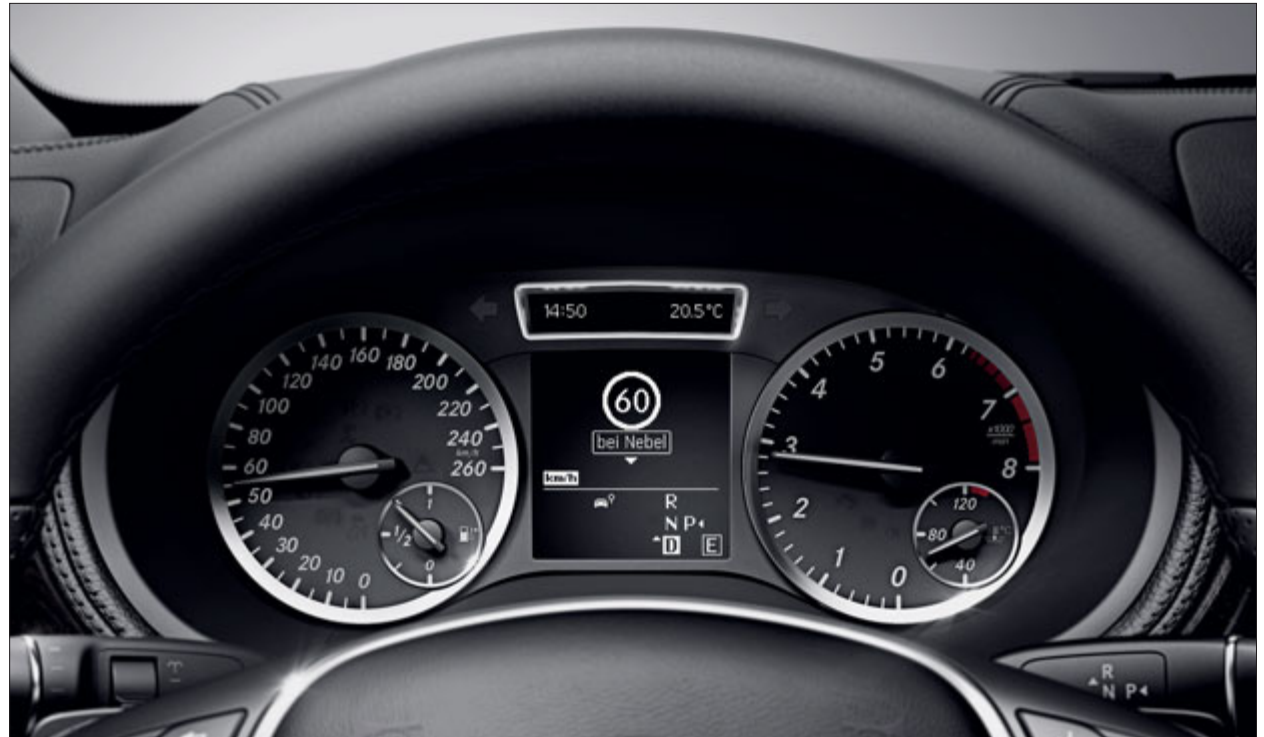
Speed Limit Assist can remind the driver about the speed limit currently in force
