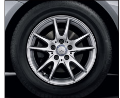
5-twin-spoke light-alloy wheels 1 , painted champion silver, with 205/55 R 16 tyres (genuine accessory, not available for Night package)
