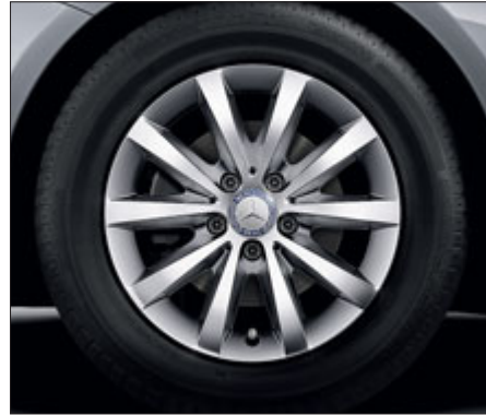
10-spoke light-alloy wheels with 205/55 R 16 tyres (optional, not available for Sports package or Night package), Code 55R
