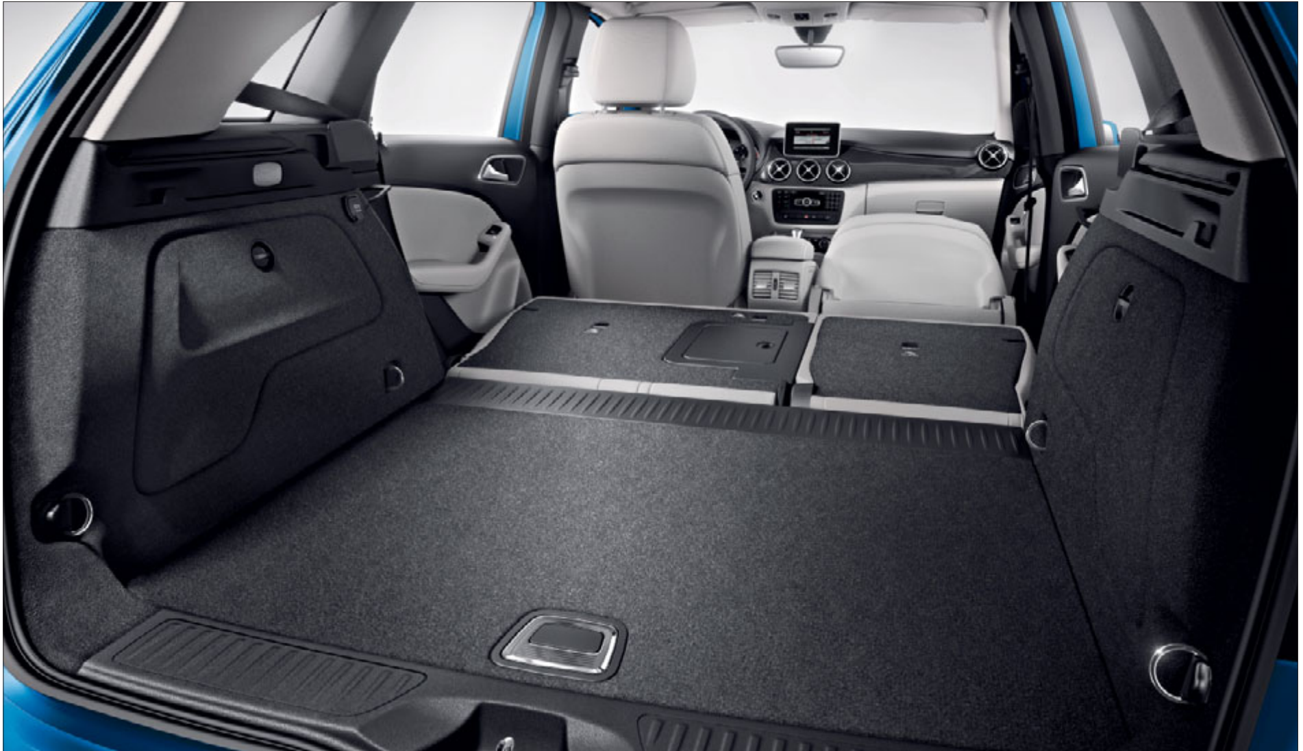
Fully folding down the rear seats produces a load compartment capacity of 1547 litres with a practically flat load area
