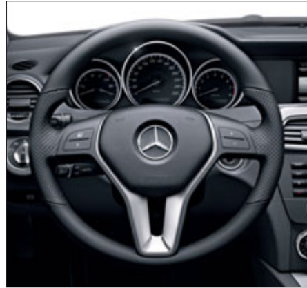
3-spoke multifunction steering wheel with 4 buttons in nappa leather, perforated in the grip area
