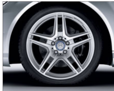
5-twin-spoke AMG light-alloy wheels with 225/40 R 18 front tyres and 255/35 R 18 rear tyres (optional, Code 786)
