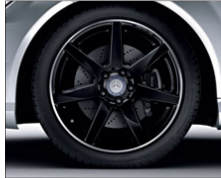
7-spoke AMG light-alloy wheels with 225/40 R 18 front tyres and 255/35 R 18 rear tyres, painted in high-gloss black and with a high-sheen finish (optional for all Sports packages and Sport models, Code 661)
