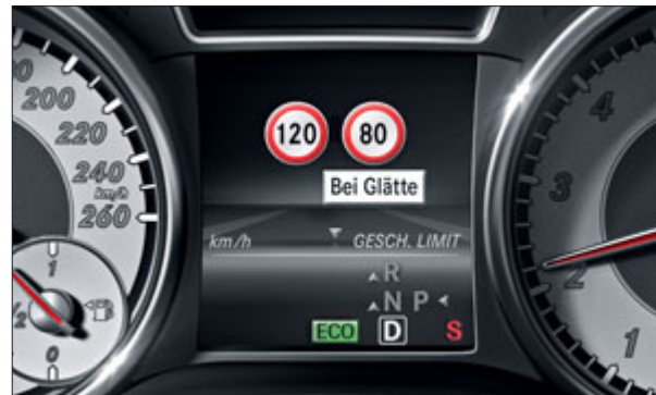
The information from Speed Limit Assist is shown both in the instrument cluster and in the COMAND Online central display
