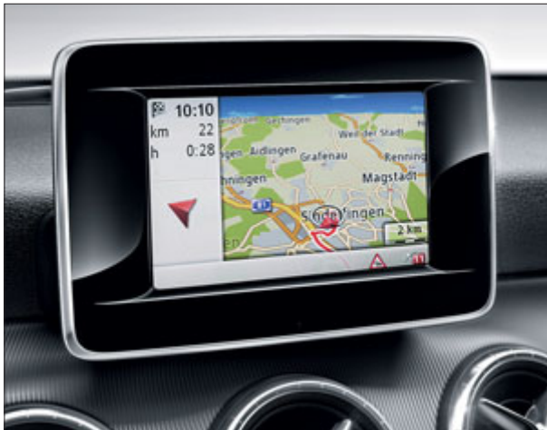
The functions provided by the Becker® MAP PILOT are indicated on the Audio 20 CD display and the TFT multifunction display in the instrument cluster
