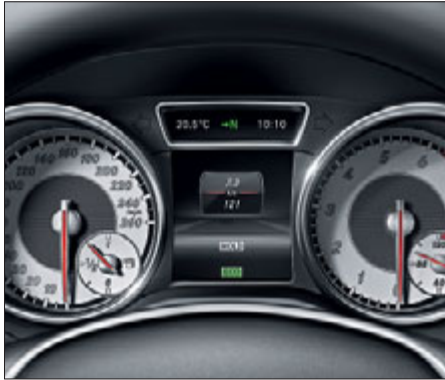
Instrument cluster in 2-tube design with colour TFT multifunction display
