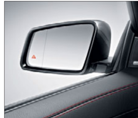
Lane Tracking package with Lane Keeping Assist and Blind Spot Assist (both also available separately)
