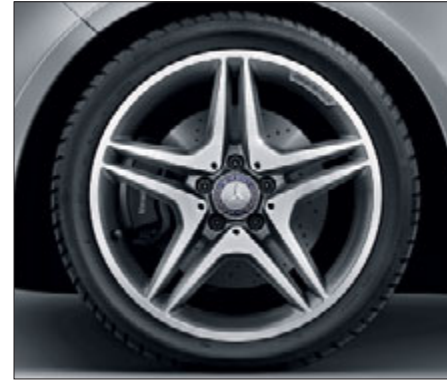
AMG 5-twin-spoke light-alloy wheels with 225/40 R 18 tyres, painted titanium grey with a high-sheen finish (standard for AMG Line, Code 794)
