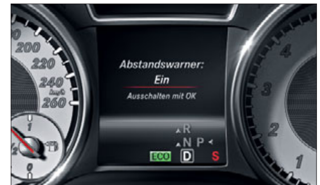
COLLISION PREVENTION ASSIST can give the driver visible and audible warnings if the safety margin is too short
