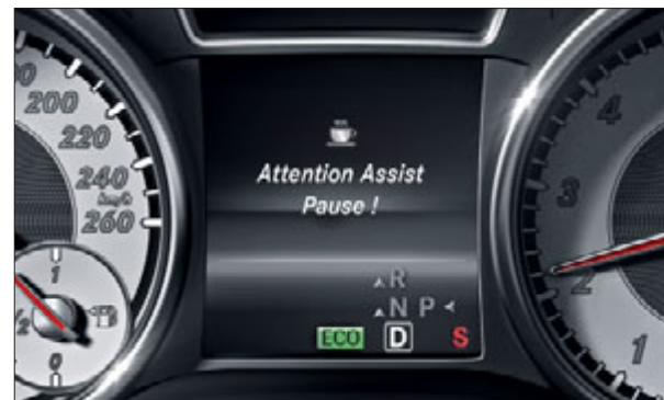
If ATTENTION ASSIST detects signs of driver drowsiness or inattention, it recommends taking a break
