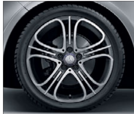
5-triple-spoke light-alloy wheels with 225/40 R 18 tyres, painted himalayas grey and with a high-sheen finish (factory-fitted accessory wheels; Code 64R) 1
