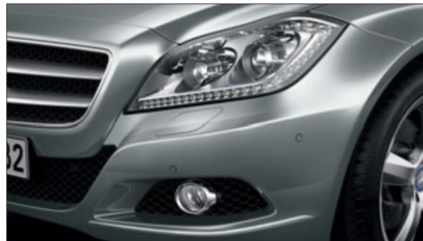
The bi-xenon headlamps with circular daytime running lamps in the bumper come as standard
