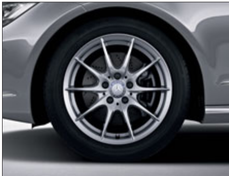
10-spoke light-alloy wheels with 245/45 R 17 tyres (standard for 6-cylinder models and CLS 250 CDI BlueEFFICIENCY Shooting Brake, optional for CLS 250 CDI BlueEFFICIENCY Coupé, Code R43)
