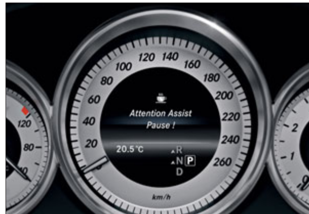
If signs of increased driver inattention or drowsiness are detected, ATTENTION ASSIST advises taking a break
