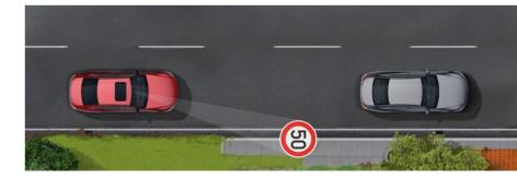
Active Speed Limit Assist adopts speed limits detected by camera or known to the navigation system as the new set speed for Active Distance Assist DISTRONIC.
