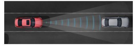
Active Distance Assist DISTRONIC and Active Steering Assist are able to maintain automatically the correct distance to vehicles ahead and to follow them, at speeds of up to 210 km/h.
