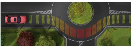
**Route-based speed adaptation** anticipates upcoming road features such as bends, junctions or roundabouts and adjusts the vehicle's speed accordingly.
