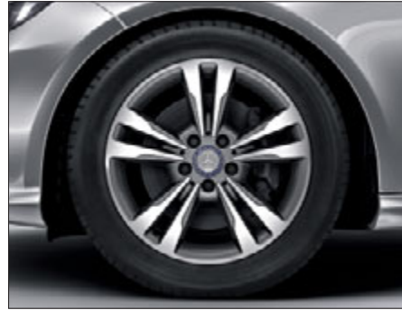
5-twin spoke light-alloy wheels with 245/45 R 17 tyres (standard for AVANTGARDE for 4- and 6-cylinder models, Code 44R/R38 2 )
