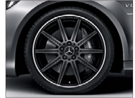
10-spoke AMG light-alloy wheels with 255/35 R 19 tyres at the front and 285/30 R 19 tyres at the rear, painted matt black, rim flange with high-sheen finish (option for AMG models, Code 752)
