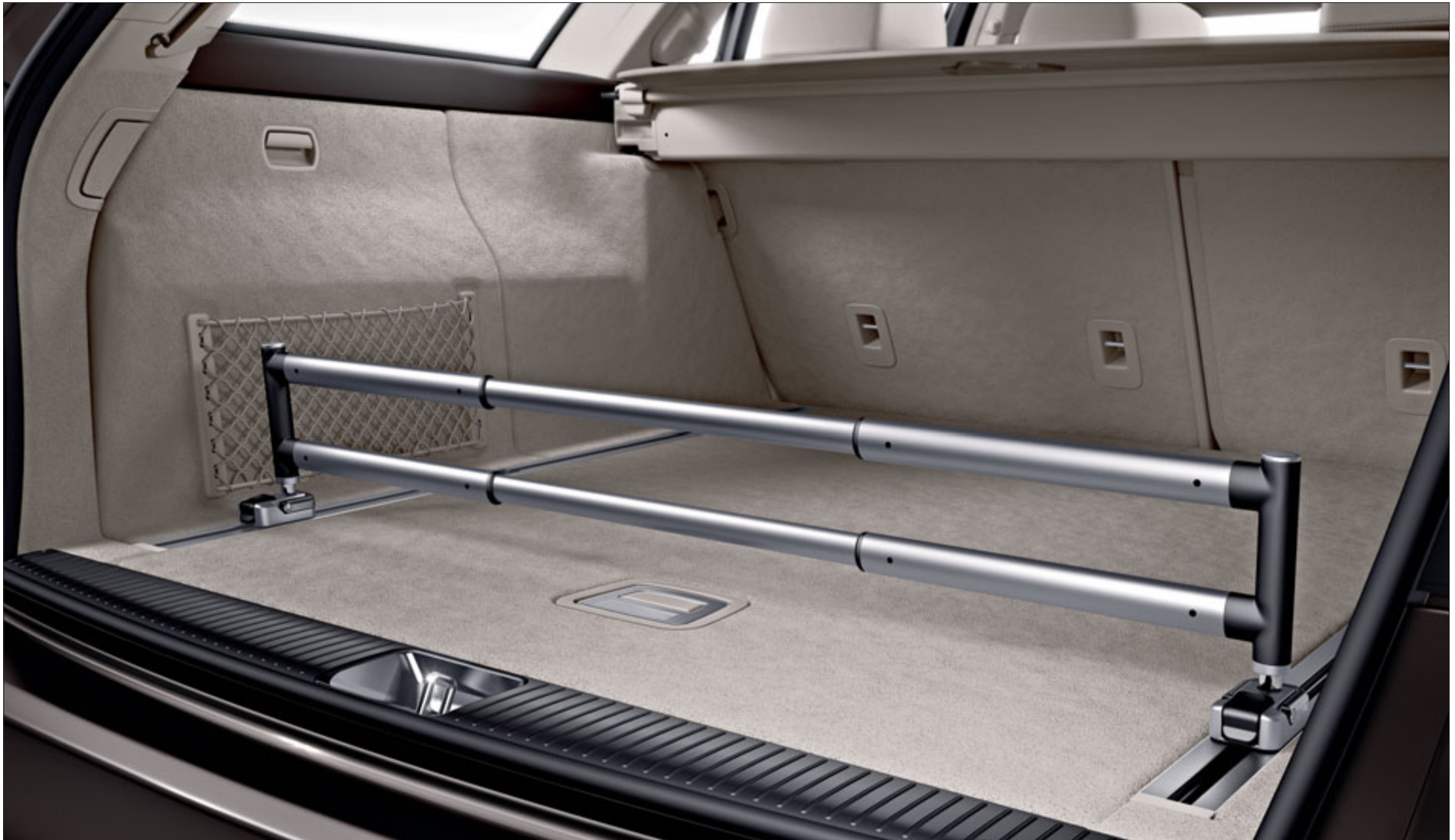
The load-securing rails in the optional EASY-PACK load-securing kit make it easy to secure the load
