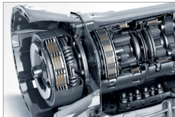
The AMG SPEEDSHIFT MCT 7-speed sports transmission
