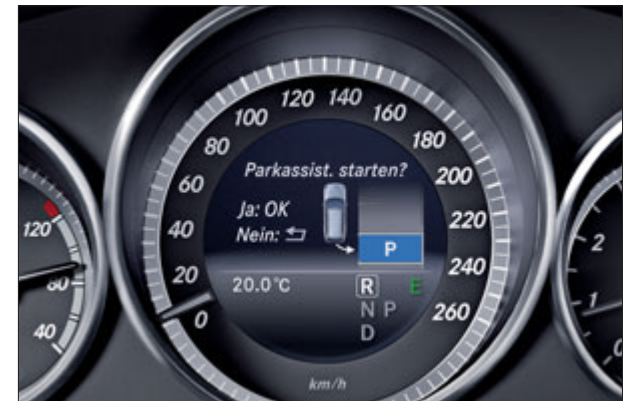
The display in the instrument cluster gives a clear picture of the parking manoeuvres at all times
