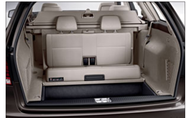
The optional folding bench seat in the load compartment can carry two people, each with a max. height of 140 cm and weight of 50 kg
