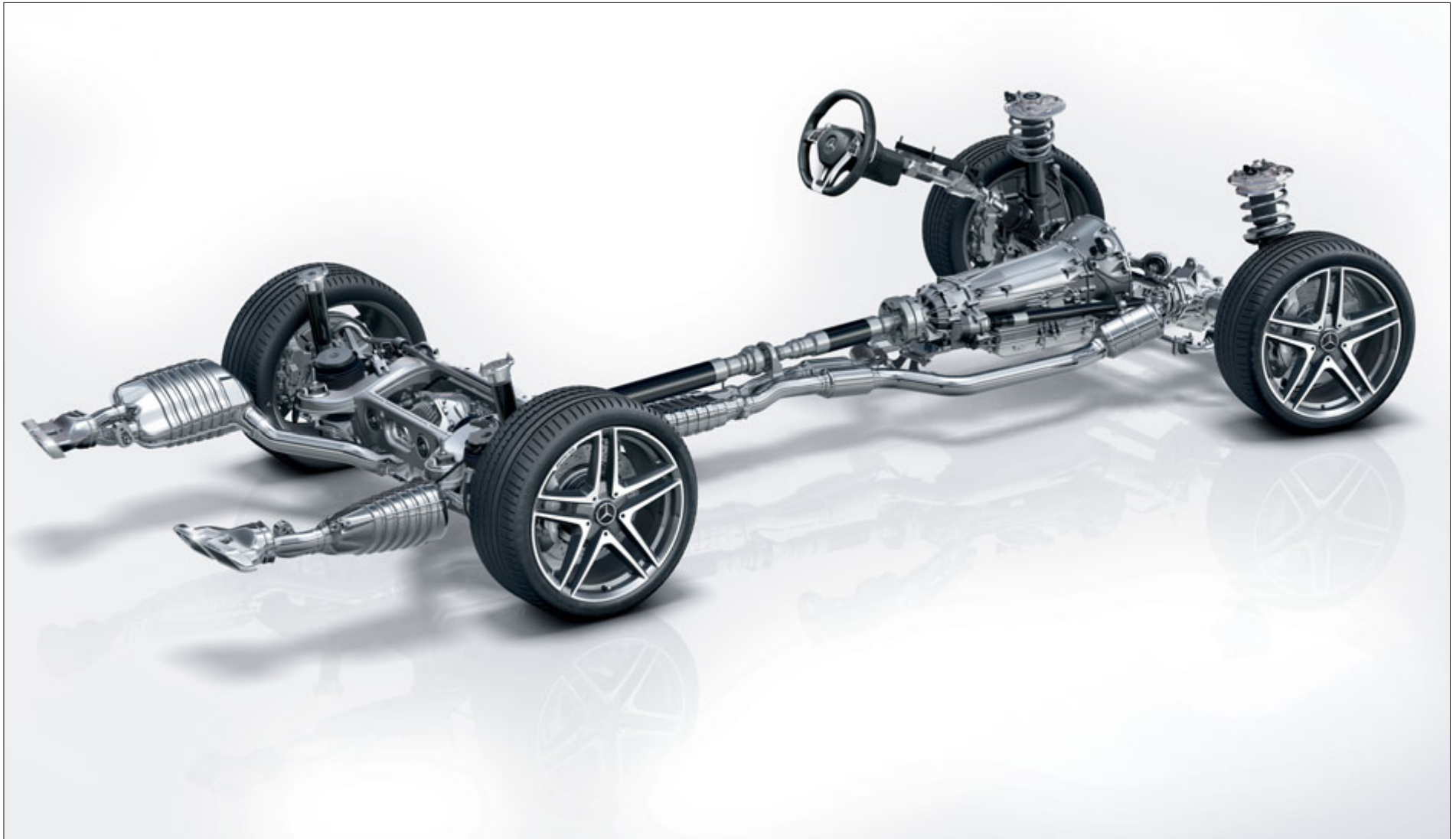
The AMG RIDE CONTROL sports suspension with a wide front axle for enhanced lateral dynamics
