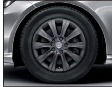
10-spoke light-alloy wheels with 225/55 R 16 tyres, himalayas grey (option for 4- and 6-cylinder models without 4MATIC, depending on the engine without extra charge, Code 55R)
