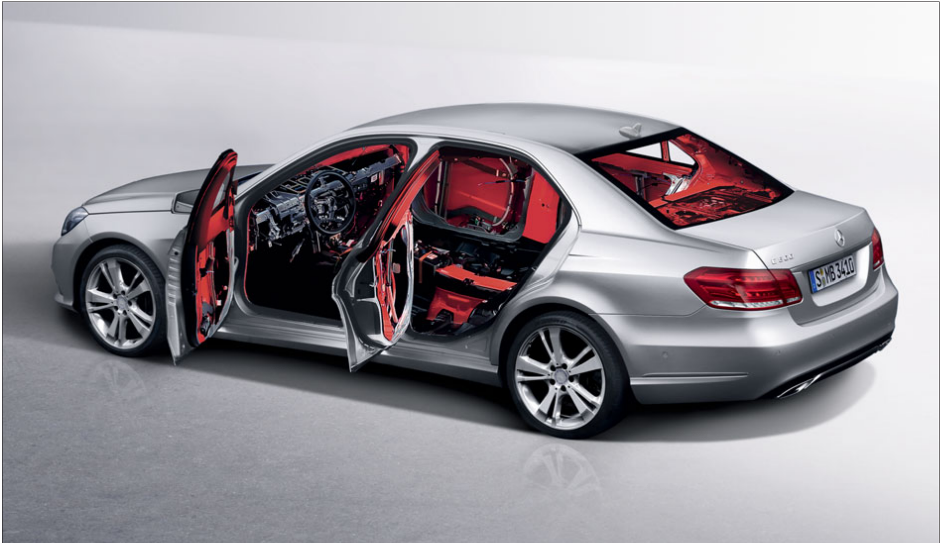
Mobile protection for extreme situations – the E-Guard: tested and certified by internationally recognised official organisations in accordance with ballistic resistance level VR4 and higher
