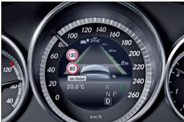
As well as speed restrictions, the Traffic Sign Assist also indicates “no overtaking” signs and “no entry” signs at motorway junctions
