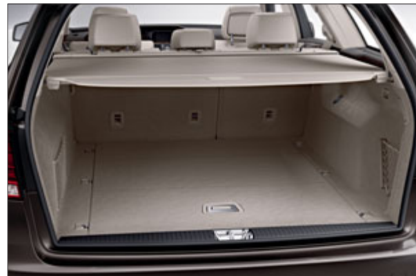
The EASY-PACK load compartment cover moves upwards with the tailgate when the latter is opened
