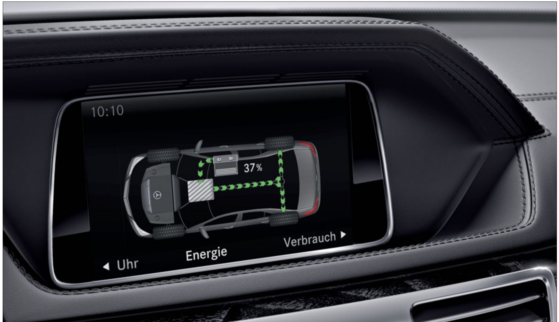
The readout on the central display provides information about the current energy flow and the battery's state of charge
