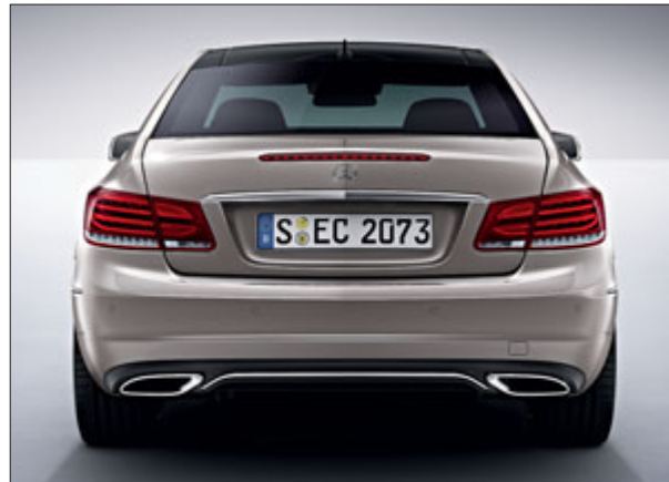
The Exterior Sports package with twin-pipe exhaust system featuring trapezoidal tailpipe trims in polished stainless steel attached to the bumper.
