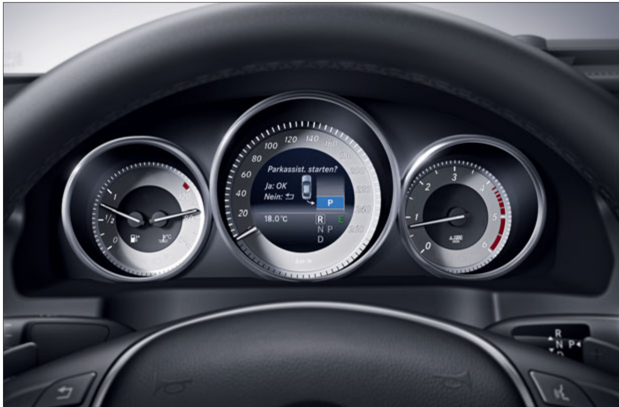
The display in the instrument cluster gives you a clear picture of the parking manoeuvres at all times.
