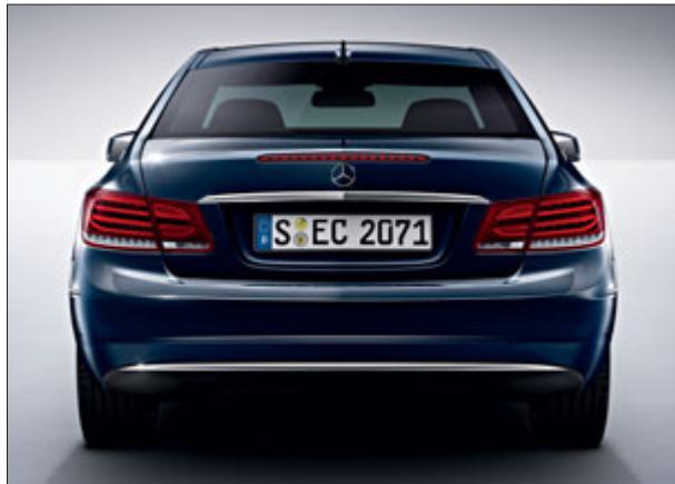
The tailpipe trims on the standard exhaust system are concealed by the new-look bumper.
