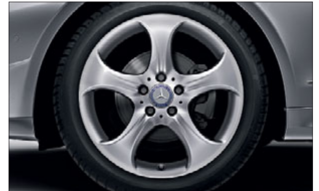
5-spoke light-alloy wheels with 235/40 R 18 front tyres and 255/35 R 18 rear tyres (optional, Code R08).
