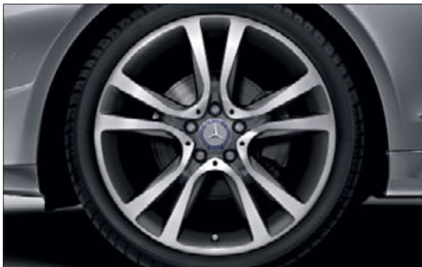
5-twin-spoke light-alloy wheels with 235/35 R 19 front and 255/30 R 19 rear tyres (optional, Code R17).
