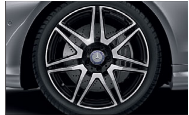
AMG 7-twin-spoke light-alloy wheels, painted high-gloss black with a high-shine finish, with 235/35 R 19 front tyres and 255/30 R 19 rear tyres (optional, Code 662, part of AMG Plus Sports package).
