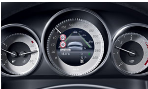
Traffic Sign Assist shows the driver the speed limits and other traffic signs currently in force on the display.
