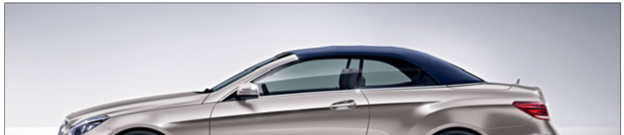
The fabric soft top can be opened and closed again easily by means of a switch – up to a speed of 40 km/h.
