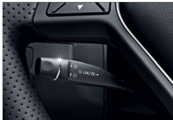
Cruise control with SPEEDTRONIC 1 variable speed limiter.
