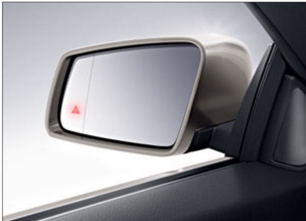
Lane Keeping Assist and Blind Spot Assist can warn the driver in potentially dangerous situations, for instance when changing lanes.
