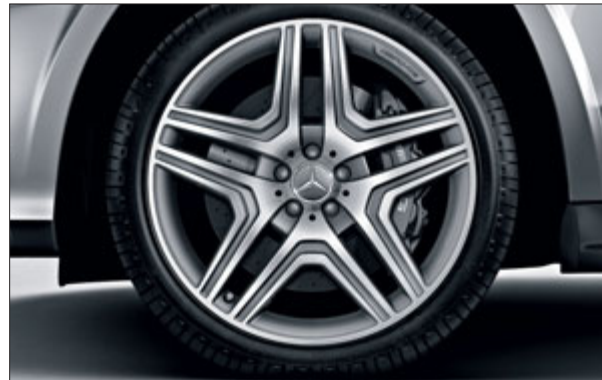
AMG 5-twin-spoke light-alloy wheel with 295/40 R 21 tyres, painted titanium grey and with a high-shine finish (option in conjunction with AMG Exterior Sports package and for GL 63 AMG, Code 798)
