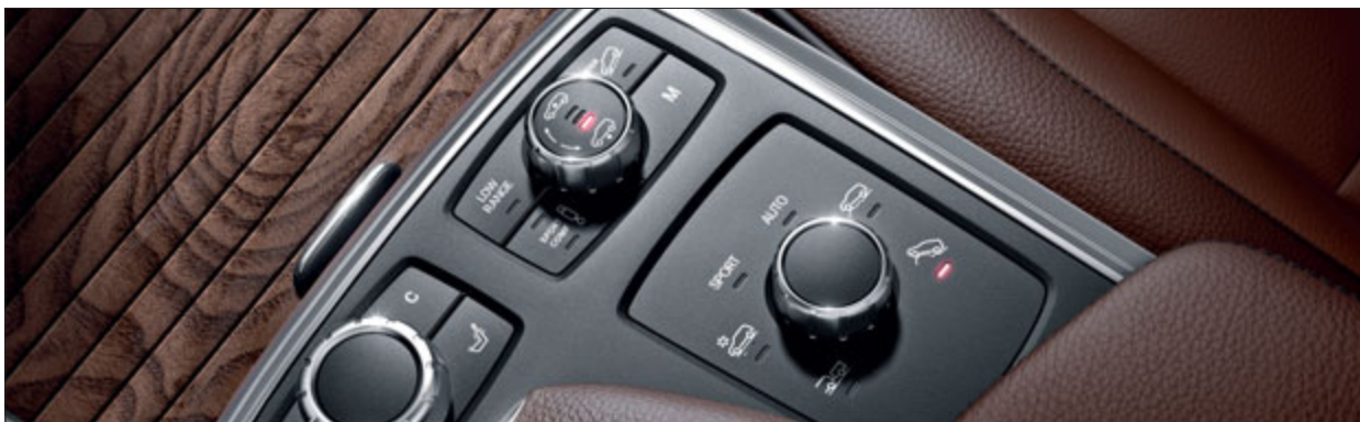
A rotary switch in the centre console is used to set the driving mode currently wanted
