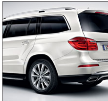
Heat-insulating, dark-tinted glass, all-round from B-pillar
