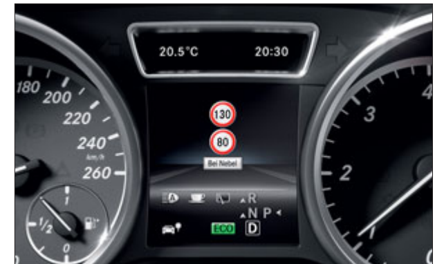
Speed Limit Assist can even indicate temporary speed limits in the instrument cluster
