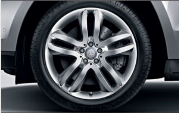
5-twin-spoke light-alloy wheel with 275/50 R 20 (option for GL 350 BlueTEC 4MATIC and GL 500 4MATIC BlueEFFICIENCY, Code R33)
