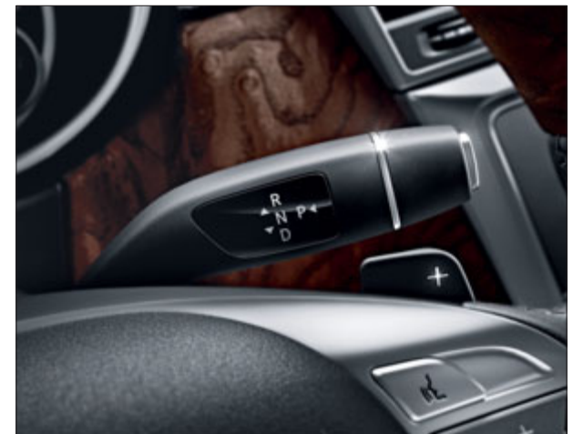
DIRECT SELECT lever on the steering wheel: the driver can intervene manually in the gear selection process via the shift paddles on the steering wheel
