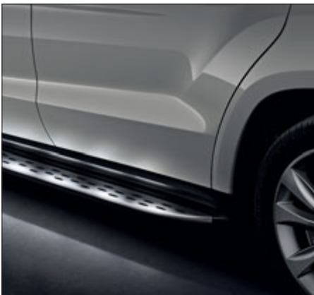
Aluminium-look running boards with rubber studs, LED illumination (standard for GL 63 AMG)
