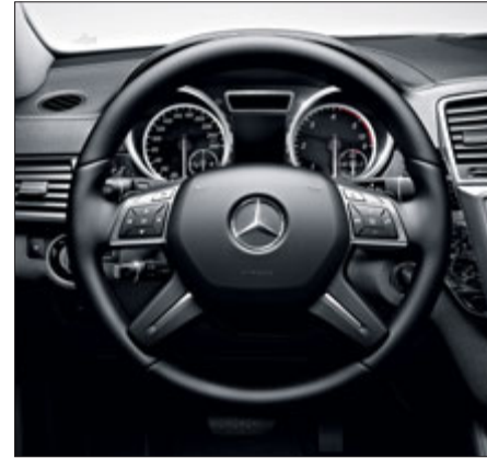
Multifunction steering wheel in nappa leather with 12 function buttons and steering-wheel gearshift paddles
