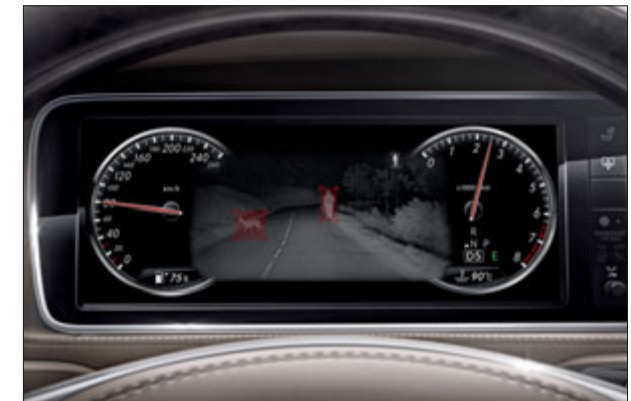
Night View Assist Plus highlights any people it has recognised and helps the drivers to react quicker to dangers by night.
