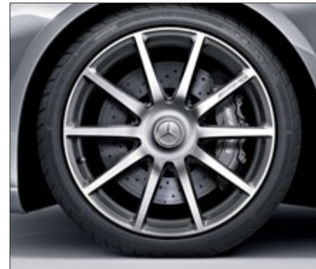
AMG 10-spoke forged wheels, painted titanium grey and polished, with 255/40 R 20 front and 285/35 R 20 rear tyres (only for S 63 AMG, S 63 AMG 4MATIC and S 65 AMG, Code 647).
