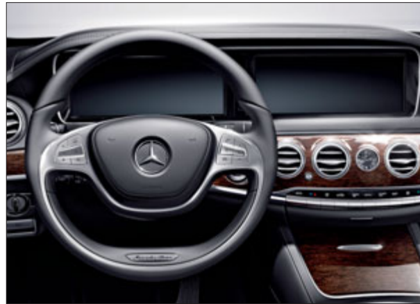
Twin-spoke multifunction steering wheel in nappa leather with 12 pushbuttons.
