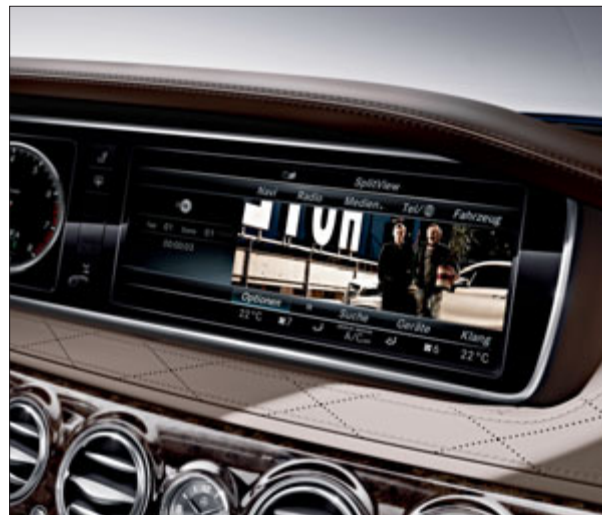
SPLITVIEW displays two different images at the same time – for the driver and front passenger – on a single screen in the centre console.
