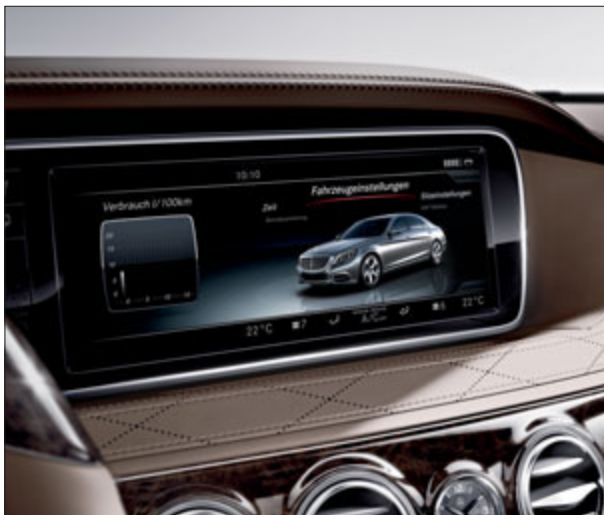
SPLITVIEW displays two different images at the same time – for the driver and front passenger – on a single screen in the centre console.
