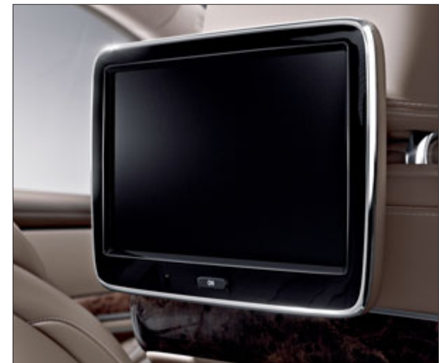
Part of the Individual Entertainment System in the rear: the 25.4 cm displays.
