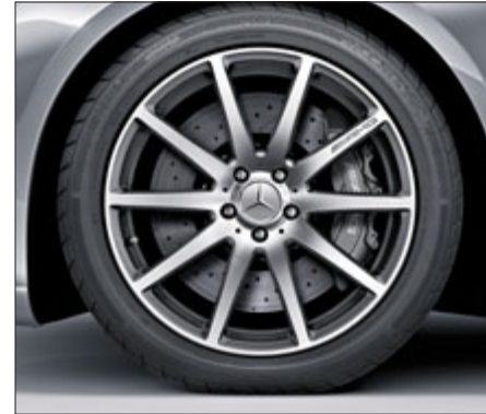
AMG 10-spoke forged wheels, painted titanium grey and polished, with 255/45 R 19 front and 285/40 R 19 rear tyres (standard for S 63 AMG and S 63 AMG 4MATIC, Code 788).
