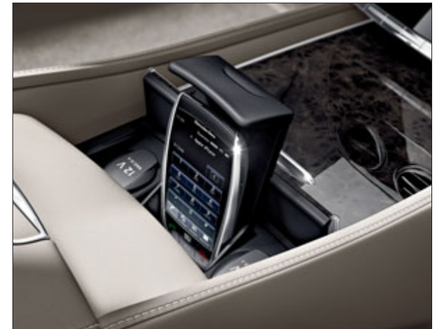
The optional handset with touchscreen serves both as a telephone and as a remote control for the seat functions of the optional Rear Seat Comfort package.
