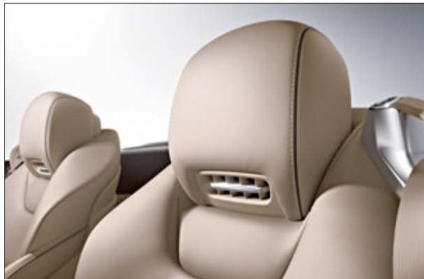
AIRSCARF delivers warm air aplenty to ensure perfect open-top motoring pleasure even in cool weather
