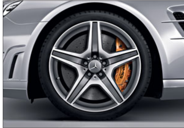
AMG 5-spoke light-alloy wheels, painted titanium grey with a high-sheen finish, with 255/35 R 19 front tyres and 285/30 R 19 rear tyres (standard for SL 65 AMG, Code 797)
