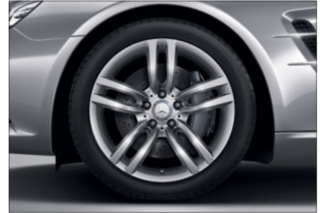
5-twin-spoke light-alloy wheels, painted vanadium silver with a high-sheen finish, with 255/40 R 18 front tyres and 285/35 R 18 rear tyres (option, Code R70)
