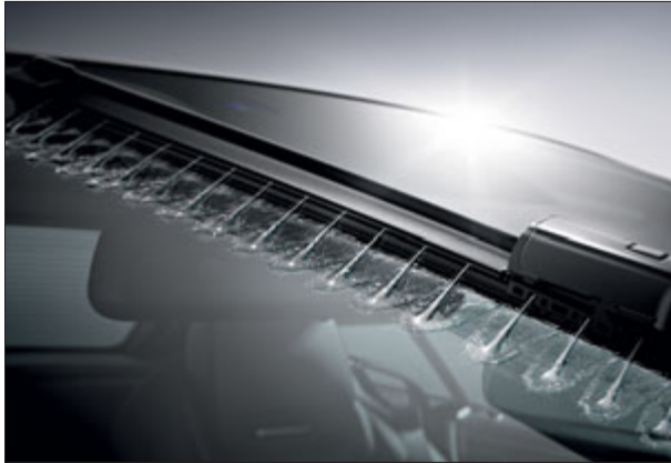
A world first: MAGIC VISION CONTROL adaptive wiper system
