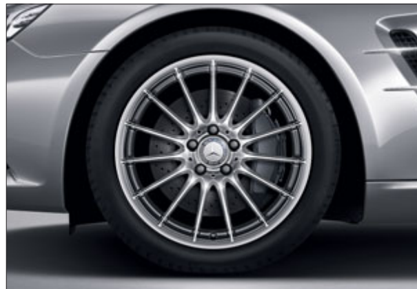
15-spoke light-alloy wheels, painted vanadium silver, with 255/40 R 18 tyres (standard for SL 500, Code R34)
