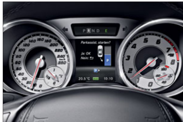
Active Parking Assist shows the driver suitable parking spaces and can carry out the parking manoeuvre automatically if required
