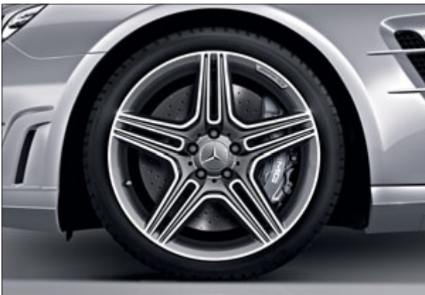
AMG 5-twin-spoke light-alloy wheels, painted titanium grey with a high-sheen finish, with 255/35 R 19 front tyres and 285/30 R 19 rear tyres (standard for SL 63 AMG, Code 793)
