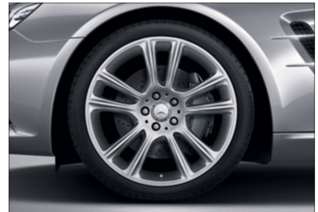
5-twin-spoke light-alloy wheels, painted vanadium silver, with 255/35 R 19 front tyres and 285/30 R 19 rear tyres (option, Code R17)
