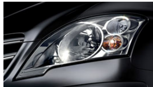
Reflector headlamps with integrated fog lights and daytime driving lights (standard on TREND)
