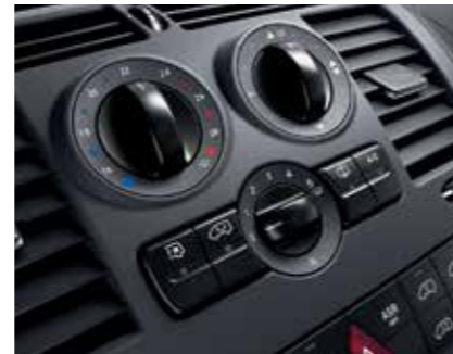
Air conditioning (TEMPMATIC).
