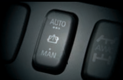
Manual intercooler water spray.
