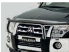
Alloy Front Protection Bar (Pedestrian safe)
