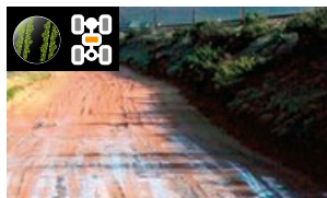
4HLC (4WD High Range with locked centre differential) For rugged terrain with low-grip surfaces.*
