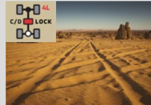
4LLC (4WD Low Range with locked centre differential) For steep hills, sand, deep snow, etc.
