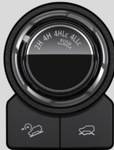
4HLC (4WD High Range with locked centre differential) For rugged terrain with low-grip surfaces.
