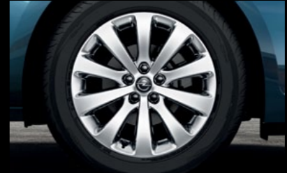
Alloy wheel, 7 J x 17", 10-spoke design, tyres 215/50R17 (with petrol) or 225/50R17 (with diesel) (PGQ). Standard on Astra Select until production Sep 7
