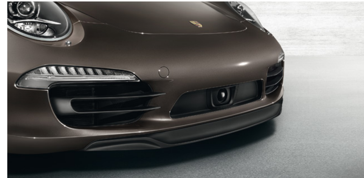
Radar sensor of adaptive cruise control
