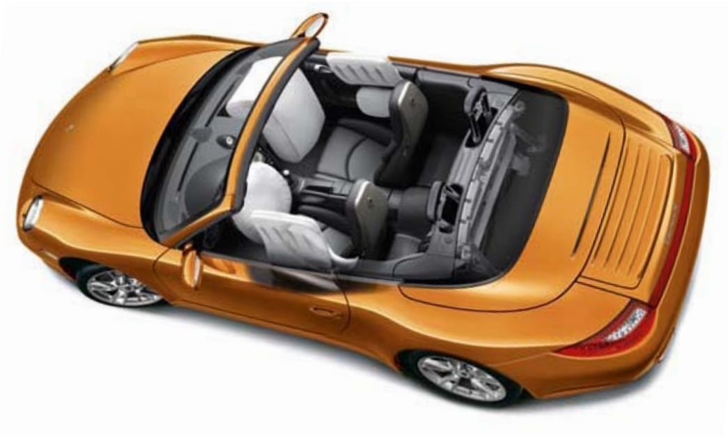
Porsche Side Impact Protection System (POSIP)
