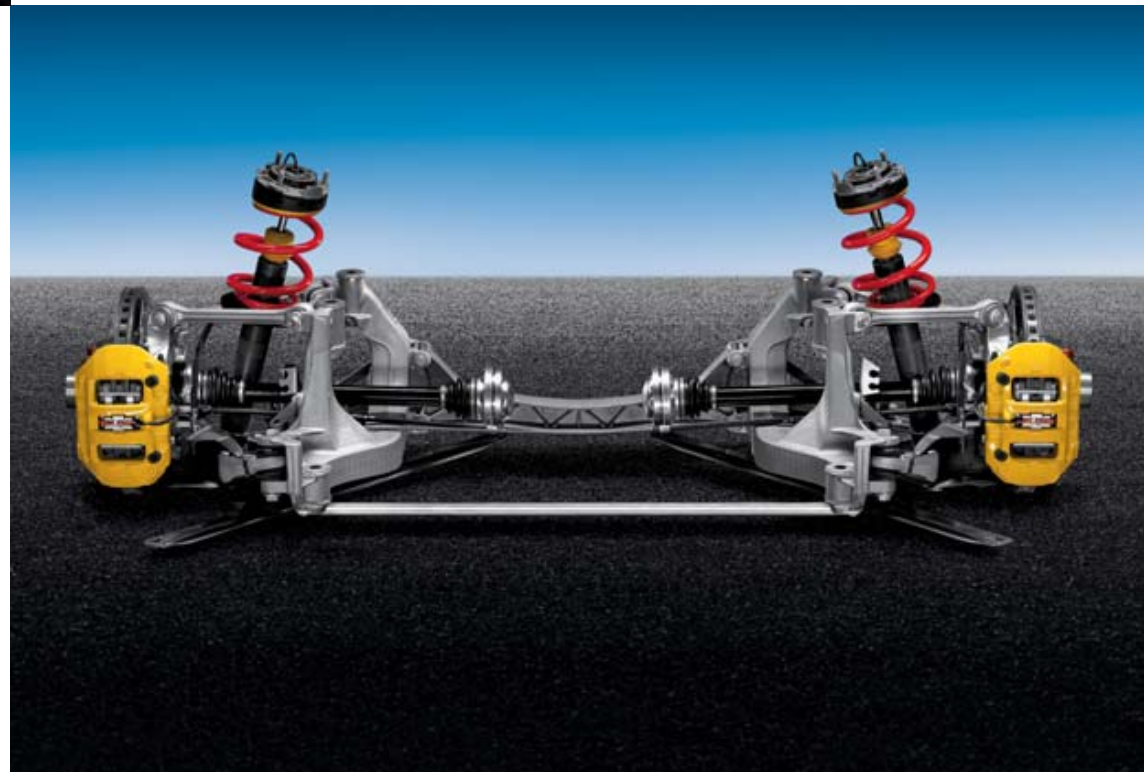
911 GT3 front axle with Porsche Ceramic Composite Brake (PCCB)
