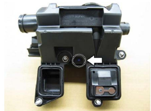
Marking on oil separator
